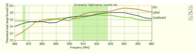
Sensitivity&Read Rang Test power: 4W EIRP
