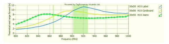
Sensitivity&Read Range Test power: 4W EIRP
