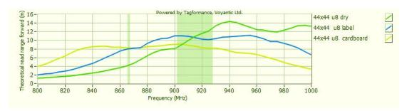
Sensitivity&Read Range Test power: 4W EIRP
